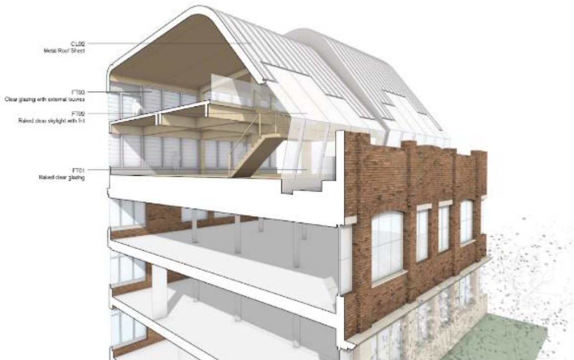
Figure 48: Section through Group 1
