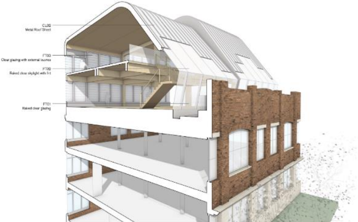
Figure 31: Section through Group 1
